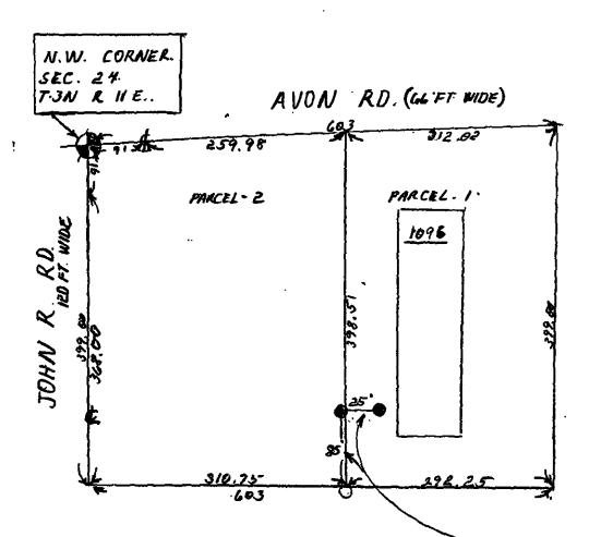
CENTERLINE OF 24 FOOT WIDE EASEMENT Note: The easement centerline may vary if field construction problems rise. Therefore, for the as-installed easement centerline call 1-800-482-7171 (Miss Dig).
