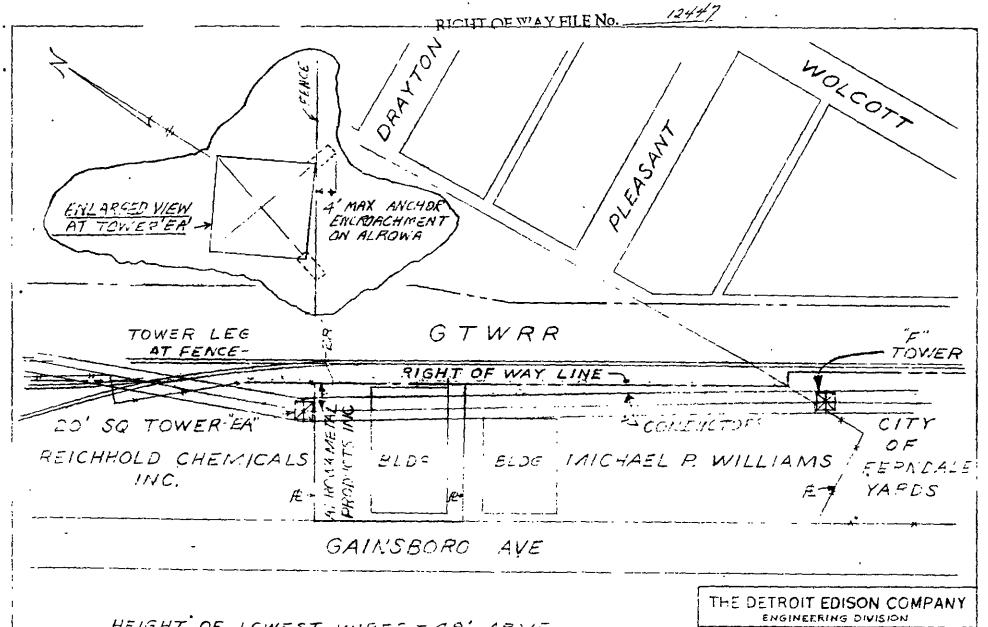
HEIGHT OF LOWEST WIRES = 48' ABJVE GRADE IN MIDDLE OF SPAN.
