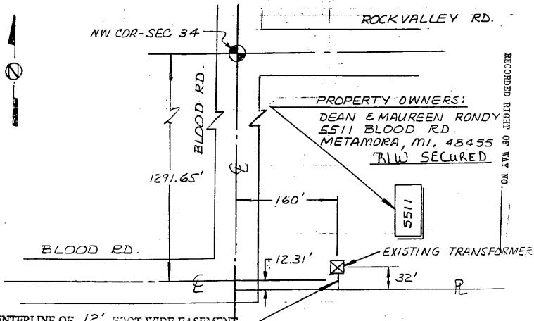
CENTERLINE OF 12' FOOT WIDE EASEMENT Note: The easement centerline may vary if field construction problems arise. Therefore, for the as-installed easement centerline call 1-800-482-7171 (Miss Dig).
