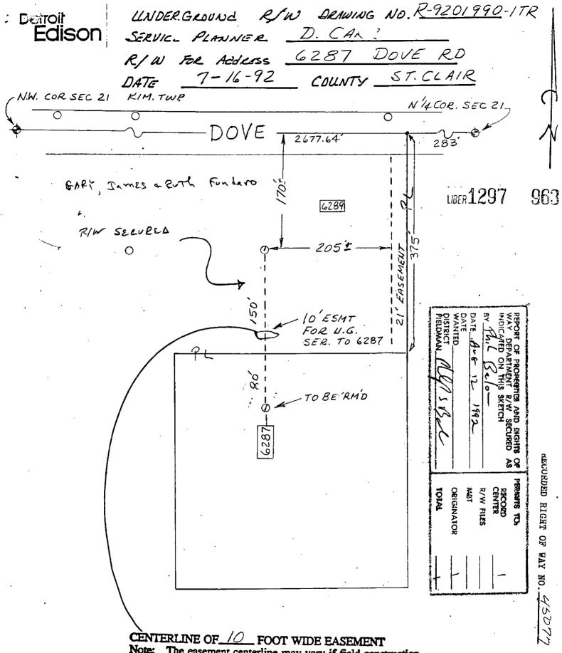
Note: The easement centerline may vary if field construction problems arise. Therefore, for the as-installed easement centerline call 1-800-482-7171 (Miss Dig).
