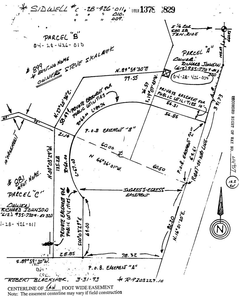
CENTERLINE OF 1/8 FOOT WIDE EASEMENT Note: The easement centerline may vary if field construction problems arise. Therefore, for the as-installed easement centerline call 1-800-482-7171 (Miss Dig).
